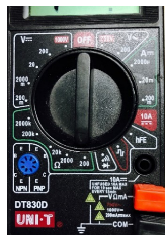
Figure 142: Select the appropriate ohm's rating
