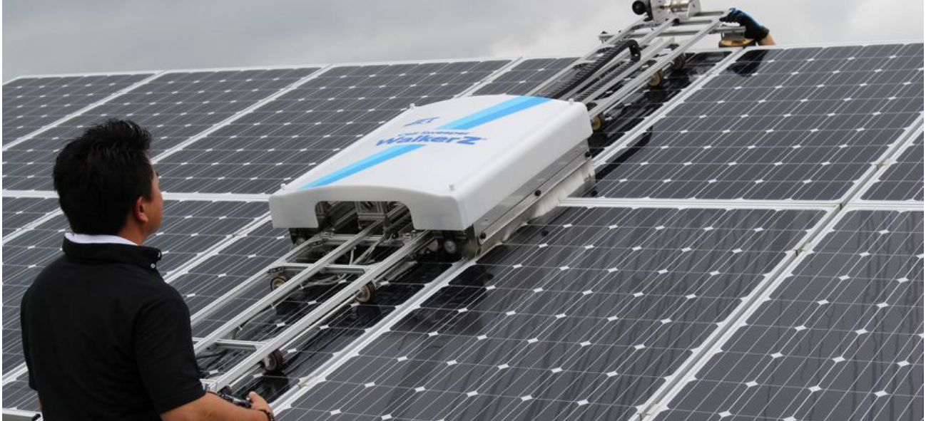
Figure 44: Wet cleaning using Robotic Method
