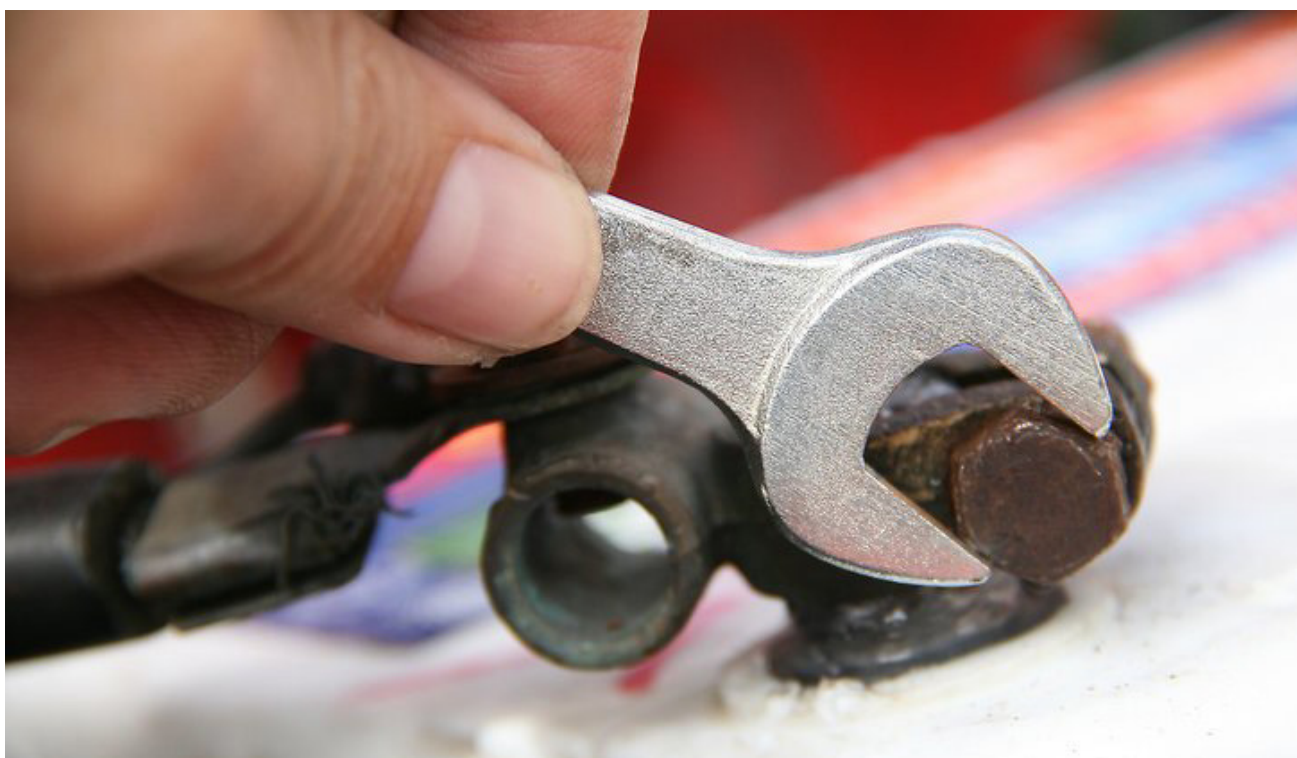
Figure 131: Tightened battery terminals
