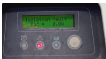
Figure 80: LED Red - Indicating incorrect operation of inverter
